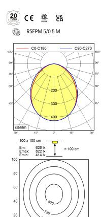
Light sourceLEDWork equipmentWithoutConnected load22 - 26 V; DCPower consumptionca. 32 W
